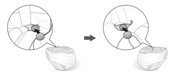
3. Locate a suitable surface on the left side of your helmet to attach the unit, clean the location with a moistened towel, and allow to dry thoroughly. Make sure that the control unit sticks on the helmet firmly. Maximum adhesion occurs after 24 hours.
