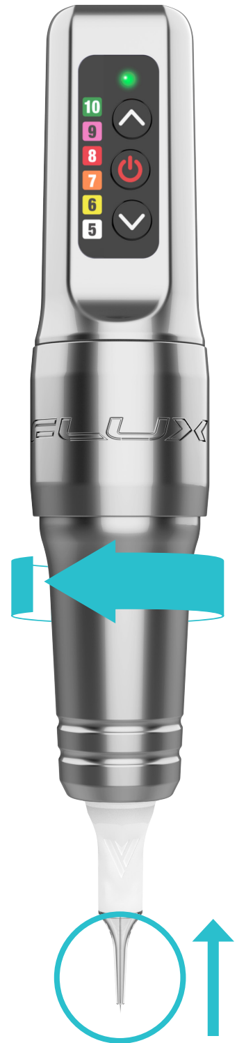
Turning the grip as shown decreases needle depth.
