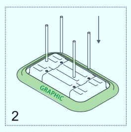
Place the vertical support poles in place firmly
