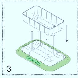
Now lift the bottom case (the one with wheels) and place on top of the support pole, fit the poles same as base
