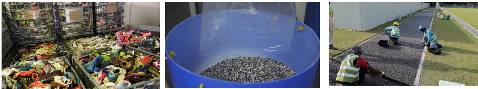
Figure 6. The sequence of sneaker recycling showing sneaker collection, shredded particles and a jogging track playground made using the recycled particles in Singapore
