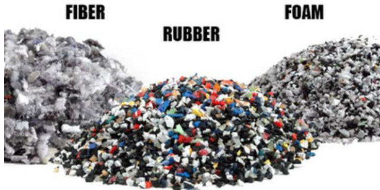
Figure 8. Small particles of footwear during the recycling process
