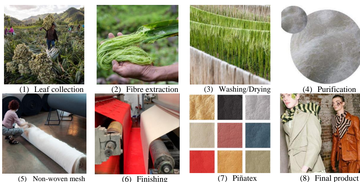
Figure 9. The Production stages of the pineapple leaf fibre-based textile
