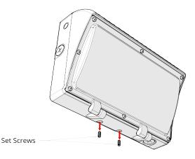
Step 1: Loosen the two (2)set screws found on the bottom of the fixture housing.
