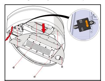
**Step 1:** With the supply power off, open the bottom cover and carefully detach the LED reflector assembly. Adjust the controller to the desired wattage by sliding the switch on the controller.
