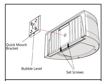
**Step 2:** Remove the quick mount bracket from the fixture and attach it to the junction box with the appropriate hardware (not included).
