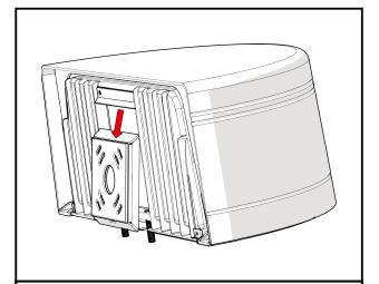
**Step 4:** Lift the fixture and tilt slightly toward the quick mount bracket. Hook the fixture housing onto the quick mount bracket as shown. Take care not to pinch any wires.
