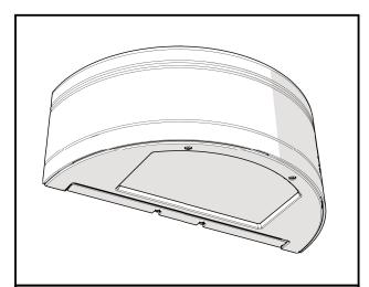
**Step 2:** Reattach the LED reflector assembly and close the bottom cover. Restore power and check that the fixture is functioning properly.
