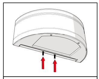
**Step 5:** Tighten the two (2) set screws to secure the fixture housing to the quick mount bracket.
