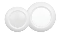
The disc surface mount LED downlight in 4 inch and 6 inch is low profiled installation solution designed to fit the tightest of spaces. The driverless DOB driver onboard technology allows this fixture to fasten to most 3 inch or 4 inch round, octagon or square junction box or shallow pan box eliminating the need for recessed housing.
