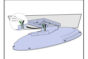
**Step 4:** Wire the supply cable from the fixture to the power source wires.
