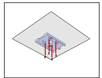
**Step 2:** Mount the bracket to the desired surface using the appropriate hardware (not supplied).
