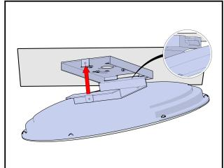
**Step 5:** Raise the fixture to secure with the locking screw removed in Step 1.
