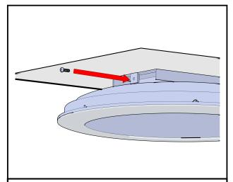
**Step 6:** Secure the bracket with the locking screw.
