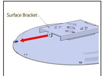
**Step 1:** Remove the locking screw to separate the top half of the surface bracket.
