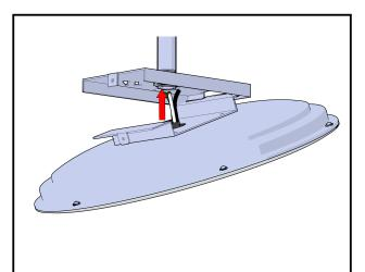
**Step 4:** Feed the supply cable from the fixture through the conduit and wire in the junction box. Black->Line; Green->Ground; White->Neutral SEE ELECTRICAL WIRING DIAGRAM ON PAGE 6
