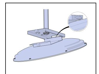
**Step 3:** Hang the fixture on the mounted bracket.
