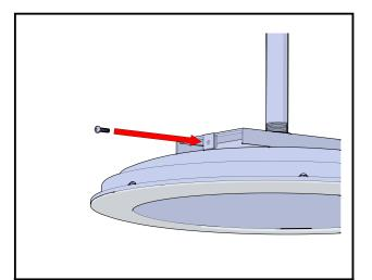
**Step 6:** Secure the bracket with the locking screw.
