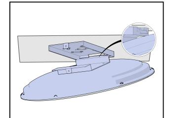
**Step 3:** Hang the fixture on the mounted bracket.
