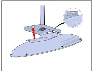
**Step 5:** Raise the fixture to secure with the locking screw removed in Step 1.
