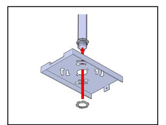
**Step 2:** Mount the top bracket to a 3/4" trade size conduit as shown and secure with two locking nuts (not supplied).
