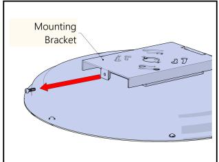
**Step 1:** Remove the locking screw to separate the top half of the mounting bracket.
