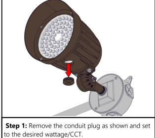
NOTE: Replace the conduit plug securely to avoid water entry into the fixture.
