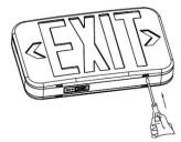
2. Knockout in back of mounting plate and push wires through the hole.
