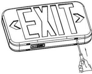
2. Knockout in back of mounting plate and push wires through the hole.
