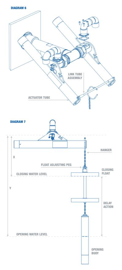
**23 OPENING WATER LEVEL (LWL)** When the actuator tube is held horizontal, the opening water level is indicated by a line on the opening buoy. Identify the desired minimum water level & measure the distance from the centre line of the valve; this is Y.
