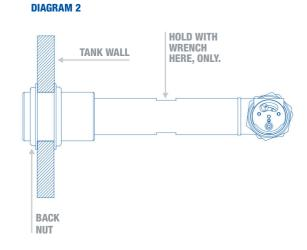
Level the two valves on the T-outlet by placing a spirit level across the T-outlet, parallel to the tank wall on which it is mounted and twisting the whole assembly to bring the valves level.
