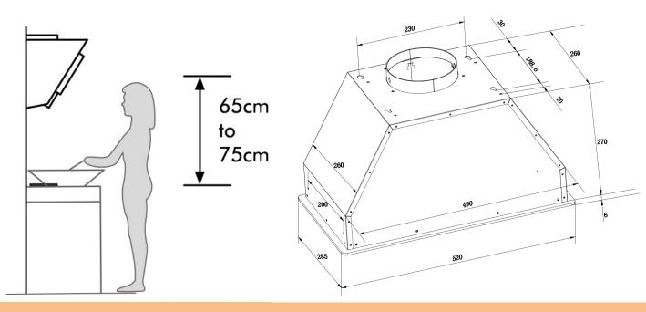
Please refer to the user manual for detailed installation and for filter replacement instructions. Insufficient distance between the cooktop and the rangehood can result in damage to the rangehood.
