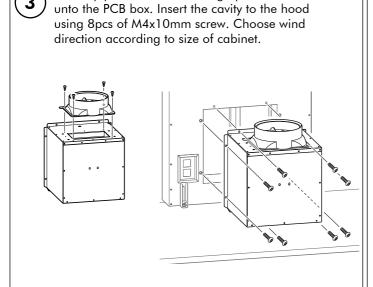
Fix the pipe on the outlet using 4pcs of ST4x14mm
