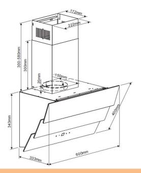
Please refer to the user manual for detailed installation and for filter replacement instructions. Insufficient distance between the cooktop and the rangehood can result in damage to the rangehood.
