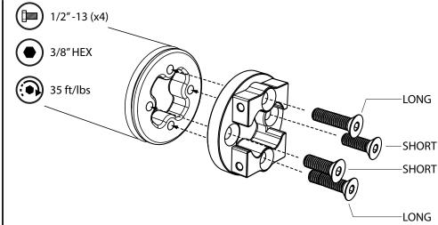
**REMOVE POLE MOUNT PLATE -** Remove the 4 bolts securing the pole mount plate. The pole mount plate has the counter sunk holes with no threads.
