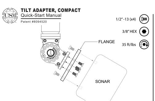
BOLT ON FLANGE - Find appropriate flange for your sonar and attach using four 3/8" HEX flat head bolts provided.
