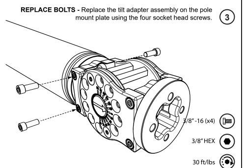
TILT ADAPTER - Remove the four flat head bolts allowing the adapter to pivot. Pivot to desired angle. Bolt holes allow 15° angle increments up to 180° of freedom. Replace bolts and attach sonar using the threaded holes.
