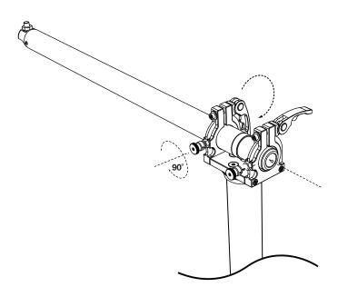
LOCK GPS POLE - After locator pin is engaged, then close GPS quick-release lever
