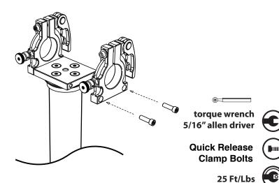
PREP GPS QUICK-RELEASE CLAMPS - Open both GPS pole clamps, pull back and turn GPS pole locator pins 90° counter clockwise
