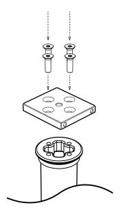
GPS TOP PLATE - Install GPS Top plate with 4 provided bolts.
