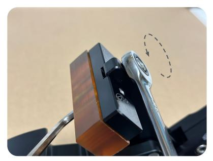
**REMOVE SHEAR BLOCK-** With the Shear Block disengaged, unthread the nut from the top of the Shear Block Carrier while counterholding the socket head bolt from the underside.
