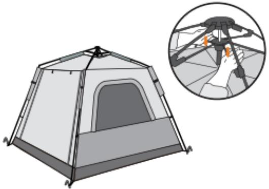
Press down the top inner supporting rods to make them stretch out and fix bottom corners with tent pegs.
