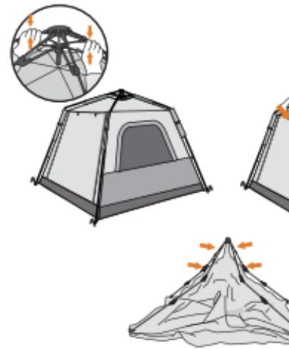
Bring the top supporting rods of the inner tent together first. Press the supporting rods inward to naturally bring them together.
