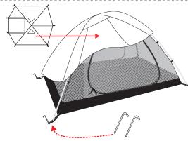
从地钉袋中取出地钉,将地钉穿过内帐底各角落的塑料环后 斜插入地面,并(如图3所示)披上外帐。 Take stake from stake bag and fix the tent with stakes
