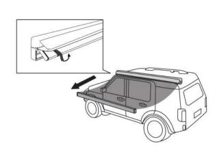
③Unzip the PVC case and undo the hook and loop fasteners.
