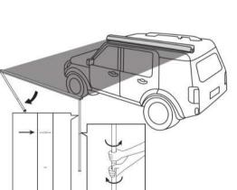
⑤Loosen the extension rod of the side awning, insert it into the corresponding mounting holes, and tighten the rod. Use hook and loop fasteners to fasten the tarpaulin to the rod.
