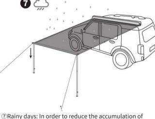
water on the roof in rainy days, please appropriately lower the height of the supporting poles to make sure the front end is lower than the height of your car so that the rainwater can flow to the ground.
