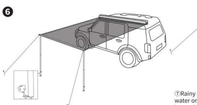
6Wind cables: Use the wind cables and stakes to ensure a steady condition of the side awning to prevent from being blown down by strong winds.
