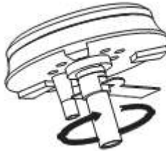
Tighten the pipe with wrench
