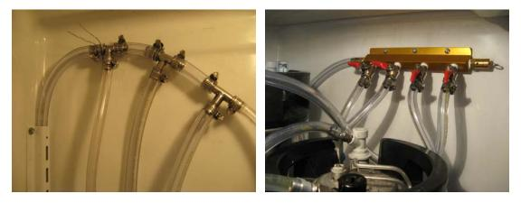
Determine where the "split" will be located, then measure from the outside regulator to the split for the first length of gas line. The rest will be 3-4 feet or 6 feet per your requirements.
