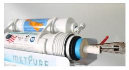
4. Insert the new membrane into the housing (o-ring end first) until you feel the o-rings seat into the opposite end cap. You may need to move the membrane in a slight circular motion to center the membrane center tube. If the membrane is not properly seated, untreated water will flow unrestricted through the system.
