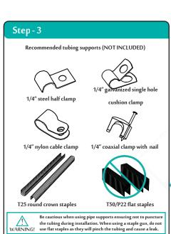
Run the tubing from shut off valve to point of use,
