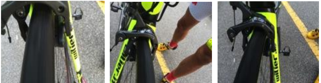
Figure 5.10 Final Check Quick Release
