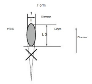
A fuselage form shall be defined as an extension or streamlining of a section. This shall be tolerated as long as the ratio between the length L and the diameter D does not exceed 3.
