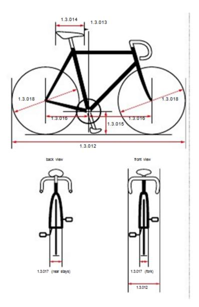
1.3.013 Only one exemption for morphological reasons may be requested; either the peak of the addle can be moved forward or the handlebar extensions can be moved forward, in accordance with Article 1.3.023.
