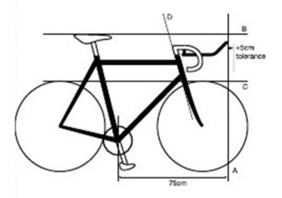
1.3.023 (a) Any device, added or blended into the structure, that is destined to decrease, or which has the effect of decreasing, resistance to air penetration or artificially to accelerate propulsion, such as a protective screen, fuselage form of fairing or the like, shall be prohibited.
