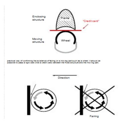
A fairing shall be defined as the use or adaptation of a component of the bicycle in such a fashion that it encloses a moving part of the bicycle such as the wheels or the chainset. Therefore, it should be possible to pass a rigid card (like a credit card) between the fixed structure and the moving part.
