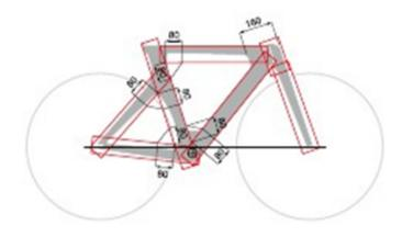
Isosceles compensation triangles with two 8 cm sides are authorized at the joints between frame elements except at the joints between the chain stays and seat stays where triangles are not authorised. Additionally, the compensation triangle between the top tube and down tube is replaced by a compensatory joint zone 16 cm wide delimited at its foremost by the front of the box for the head tube.
