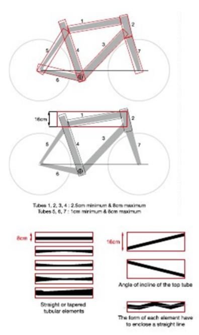
1.3.020 For road time trials and for track competitions, the elements of the bicycle frame may be tubular or solid, assembled or cast in a single piece in any form (including arches, cradles, beams or any other). These elements, including the bottom bracket shell, shall fit within a template of the "triangular form" defined in article 1.3.020. (See diagram "Shape (2)").
