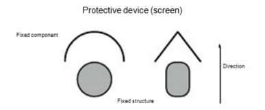
A protective screen shall be defined as a fixed component that serves as a windscreen or windbreak designed to protect another fixed element of the bicycle in order to reduce its wind resistance.
