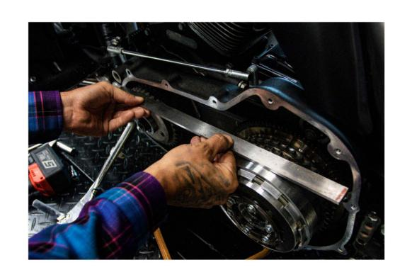
2. We recommend installing the clutch basket and the sprocket assembly using tapered torx compensator bolt H-D part #10500031 and the oil slinger washer supplied in the kit, there should be NO endplay on the motorsprocket.
