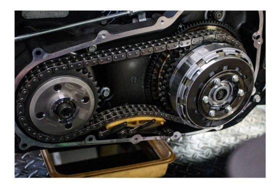
5. Verify that the threads are clean on sprocket bolt and clutch nut and prime, install using Loctite Thread Locker 262 Red. Torque the motorsprocket bolt (with supplied oil slinger) to 175 ft/lbs. Torque clutchhub nut to OEM specs per manual.
