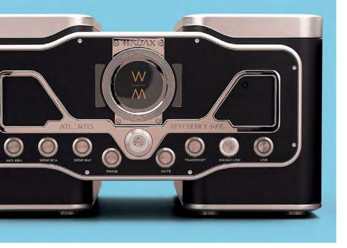
conventional single-cable interface (SPDIF and AES/EBU) carries a single signal that emerges the left channel, right channel, and clock. The clock must then be recovered from the signal at the DAC, where it becomes the timing reference for the DAC. This recovered clock is prone to jitter, or timing errors. It's a far better approach for the DAC's clock to be the timing reference, with the source component locking to that clock.
