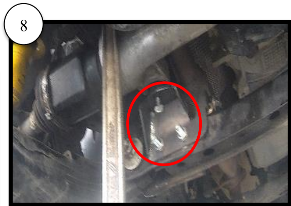
Fitting New gear bracket. (Right Side) ( E ) (Should have tool for help push) ( Hex Nut+M10x1.5+WS )
