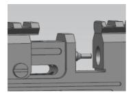
To insert the magazine, pull a pistol slide back to open the bolt
