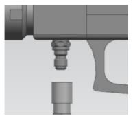
Put in a coupler supplied with gun together
