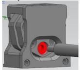
If Pellet inserted but not properly Seated, Press the tip of a ballpoint pen into pellet's skirt to properly seat
