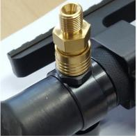
Attach the hose from your fill device to the Rex-FA adapter.
