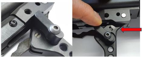
It has automatic safety lock on the under lever. So, pull the safety lock for releasing when under lever return to shot position..
