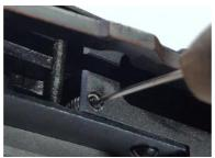
Using a 0.89 mm Allen key, turn the screw clockwise to decrease trigger pull weight and counter-cockwise to increase trigger pull weight.
