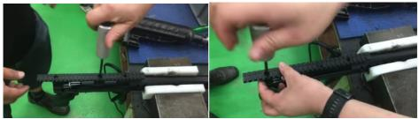
Take out mounts with releasing two screw
