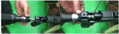
Put & turn cylinder in and keep 0.5mm~1mm gap between barrel and valve.
