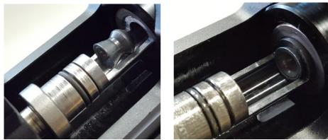
Insert pellet and push pellets to breeze of barrel & properly seat pellet. If the pellets skirt is not flush with the barrel the accuracy will be poor.
