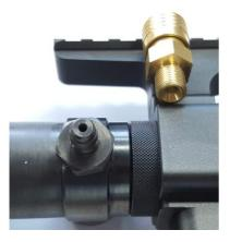
The REX-FA uses a fill adapter (included). Do not use any other type of adapter other than the one included with the gun!
