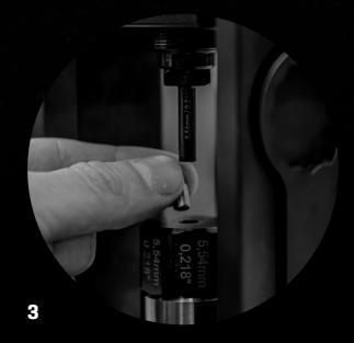
Insert the lead cylinder into the pressing mold and press the lead cylinder by moving the lever all the way down.
