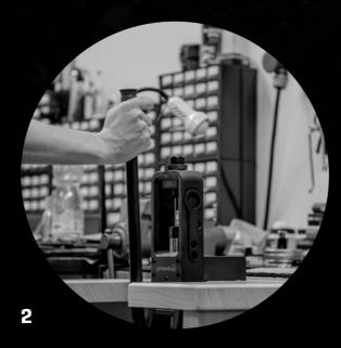
Move the lever towards you and keep it in the middle position so that there is a room for the lead cylinder in the pressing mold.
