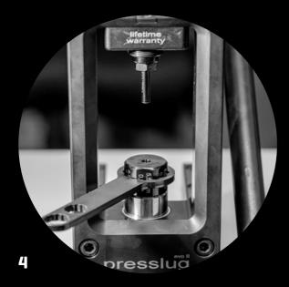
Screw the pressing mold in your desired caliber into the press and tighten it with the included mounting key. Loose mold might cause deformations of the slug.
