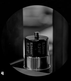
Return the lever all the way back to the upper position. The needle will push the completed slug out of the pressing mold.
