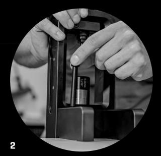
Secure the press on the table with the supporting bars and the supporting plate. You are going to have to drill four holes into the table. The working area must be flat and stable.
