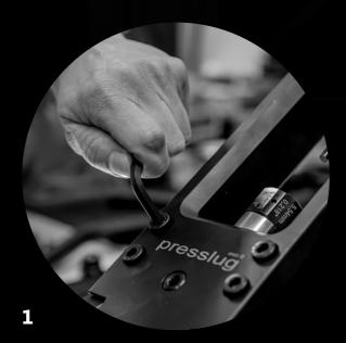
Attach the supporting bars to the press with four screws.
