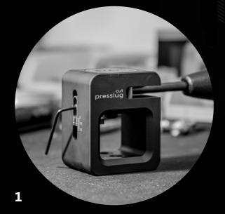
Set the desired height of the lead cylinder on the scale. Use an Allen key to tighten it.
