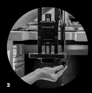
Attach the lever to the right or the left side of the press and secure it in place with the included 24 mm key.
