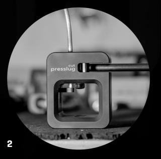
Insert the lead wire into the opening on the upper side of the cutter. The end of the wire must touch the scale.
