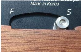
In addition to the safety catch, a loaded and cocked rifle can be made safe by decocking (uncocking). To decock the rifle, first pull the sidelever back to the rear position and remove the magazine. While holding the sidelever, squeeze the trigger and let the lever return forward under your control. The rifle is now decocked
