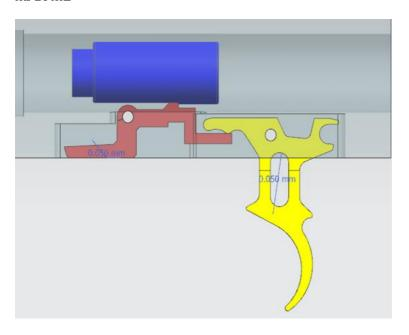
First-stage Move 2 degree Sear and 5 degree trigger blade.
