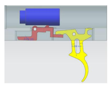
Two -stage Move 6 degree Sear and 10 degree trigger blade.
