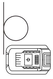
Recharge discharged batteries as soon as possible after use or battery life may be greatly diminished. For longest battery life, do not discharge batteries fully.
