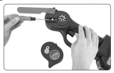
Step 5 Install the guide plate and new chain and notice the direction of the chain.
