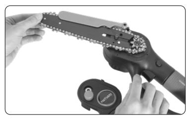
Step 6 Adjust the tightness of the chain.
