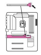
**Insert the graphics** card into the primary PCI-e slot on the motherboard. Press firmly until you hear or feel a slight click.
