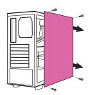
Remove the screws in the case where you will be placing the graphics card.
