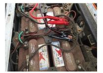
For a more permanent connection attach the ring terminal cable. The cable and Anderson quick plug can stay located in the Golf Cart battery storage compartment. The quick plug extension cable would be used to move the Hurricane up to 25 feet away if needed.
