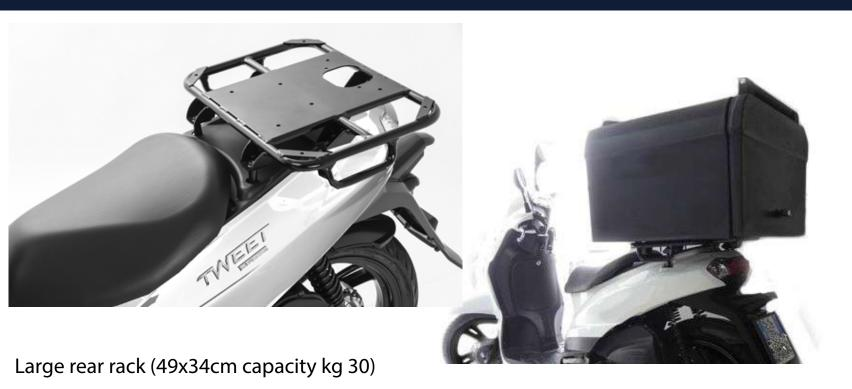
It is possible to combine a 140-liter maxy box with flap opening e door lock. External dimensions (mm) 600x633x467, opening 520x360, internal 520x480x360
