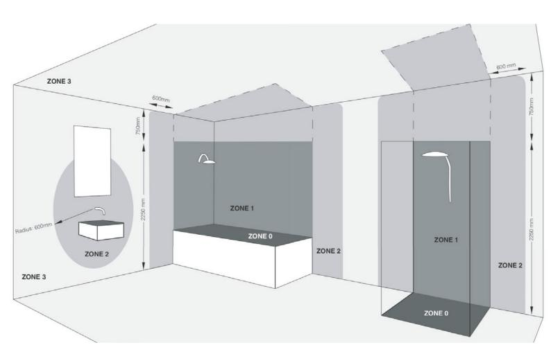
The following information is a guide to help you understand what fittings can be placed in a bathroom. This is not an installation guide and reference should be made to the IEE Wiring Regulations (17th Edition) or a qualified electrician.
