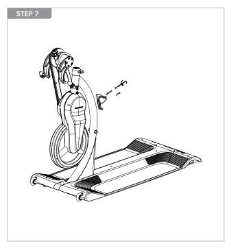
Attach water bottle cage to center upright frame with 4mm allen key wrench using item 4-socket head cap screws.
