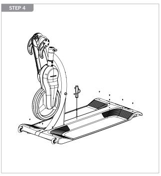
Secure BASE PLATE to BASE FRAME from step 3 with item 3-PHILLIPS HEAD SCREW and PHILLIPS HEAD SCREW DRIVER.
