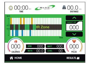
In the heart rate control workout, you may press Up/Down ( $\land/\checkmark$ ) keys to adjust the target heart rate setting. The target heart rate zone (+, -5bpm) will be highlighted and your heart rate progress will be illustrated on the profile display. The pulse data display window will show the actual heart rate.
