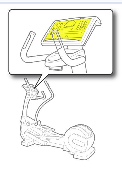
**Control panel**: controls all available functions, from setting up workout programs to viewing messages and related workout information.
