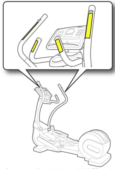
**Sensors**: **levers** and **fixed handles** have sensors for monitoring the heat rate (hand sensor), in the 700 and 700 SP versions of the equipment.
