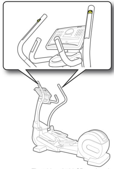
**Levers**: these can be grasped by the user to perform the exercise with arm movements. The 700 and 700 SP versions have **sensors** for monitoring the heat rate (hand sensor) and the **Fast Track Control** to change the effort level.
