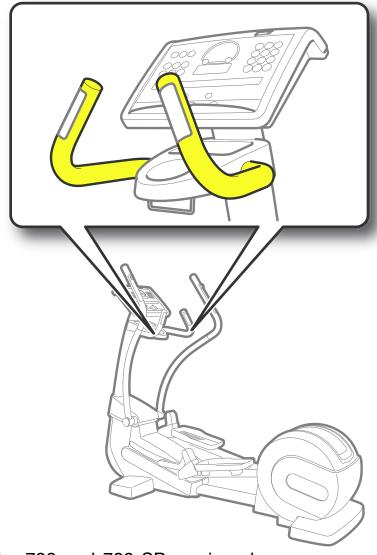
**Fixed handles**: these can be grasped by the user during the workout. The 700 and 700 SP versions have **sensors** for monitoring the heart rate (hand sensor).
