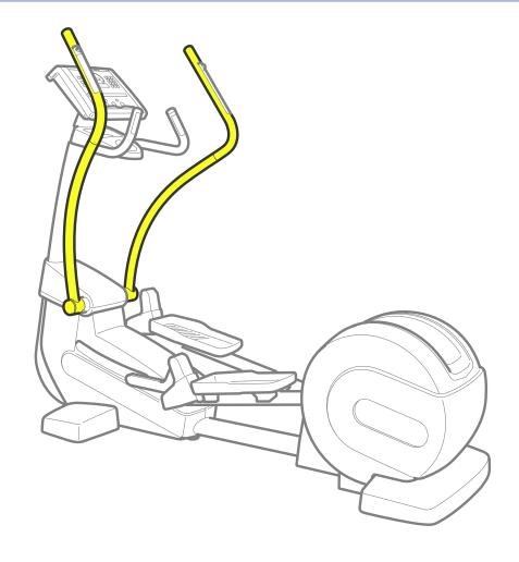
**Levers**: these can be grasped by the user to perform the exercise with arm movements. The 700 and 700 SP versions have **sensors** for monitoring the heart rate (hand sensor) and the **Fast Track Control** to change the effort level.
