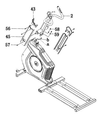
3. 3. Take out the console 44, connect the aluminum back cover 61 with the vertical tube set through screw 56, and thread the power plug c out of the hole; connect plug c and d; Connect the aluminum back cover 61 with the console with screw 60.
