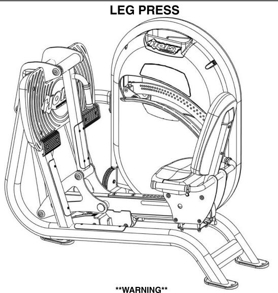
TO PREVENT POSSIBLE TIPPING, BOLT THIS UNIT TO THE EXERCISE FLOOR USING MINIMUM 4-1/2" LONG BOLTS. FAILURE TO DO SO MAY RESULT IN SERIOUS INJURY OR DEATH!
