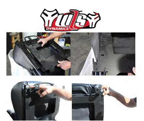
Step 6: Repeat for other seat. Reattach seat belts to seat frame as shown with nuts and bolts.
