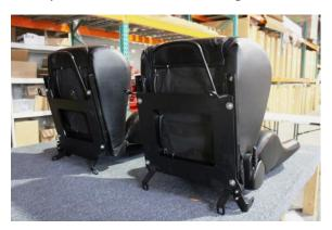
Step 7: Using factory seat bolts, reattach seat to floor.
