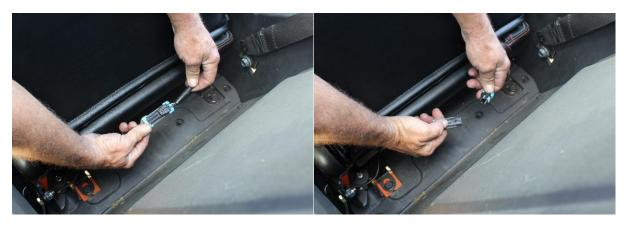
Remove seatbelt latch bolted to the seat using socket wrench.
