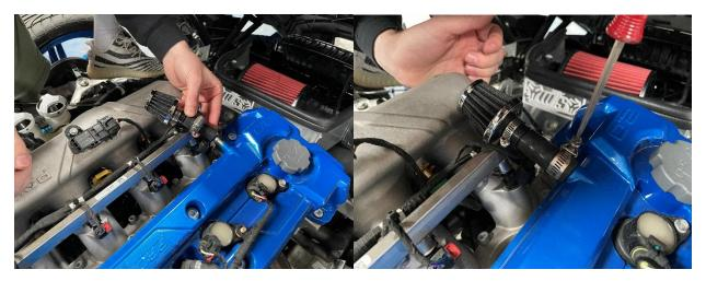
9.) Install your newly assembled Extended Small Filter Kit by sliding the open end of the kit down onto the nozzle that is protruding from the valve cover. Then, tighten the 1" hose clamp down using a flathead screw driver to secure kit to valve cover, as shown above.
