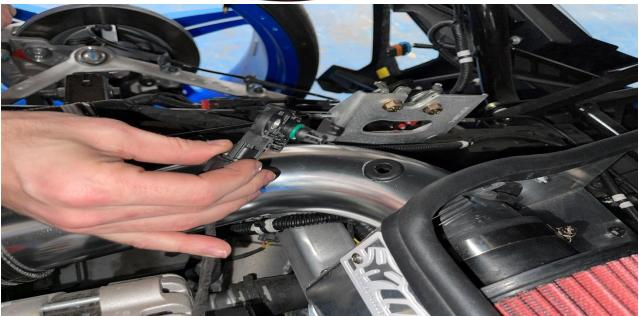
7.) Next, insert your O2 Sensor into your Large Cold Air Tube with Rubber Gasket on 90-degree Bend.
