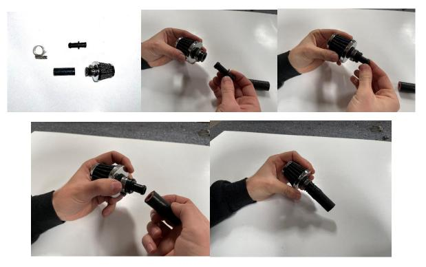
8.) You are then going to want to install your Valve Cover Filter Extension Hose and the Small Valve Cover Filter together using the stock Double-
