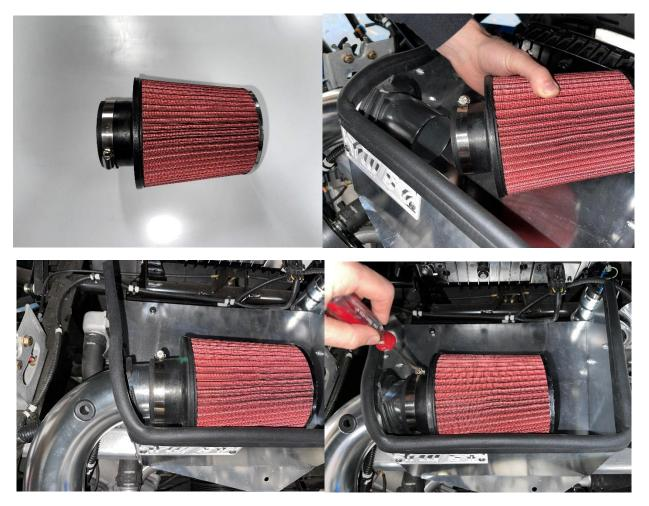
6.) Your next step is installing your Large Filter. As shown above, make sure the filter sits comfortably in the tray as well as proportionally around the circumference of the end of the Large Cold Air Tube with Rubber Gasket on 90-degree Bend. Once your happy with the fitment, tighten your final large 3-4" hose clamp.
