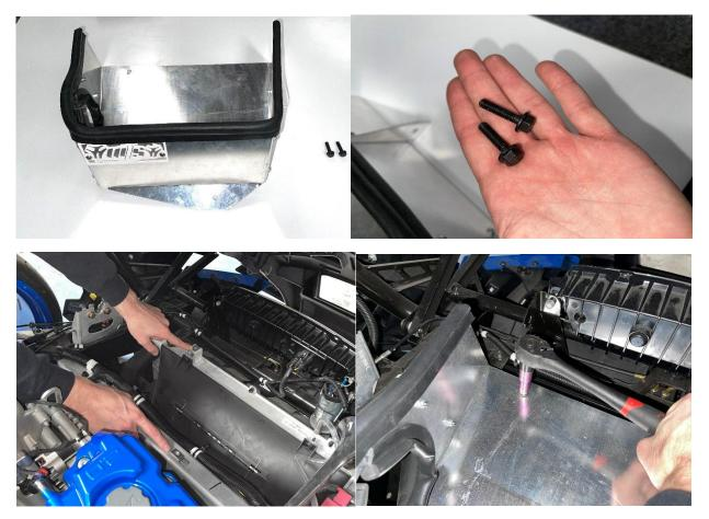
3.) For the next step, using your **2020 Cold Air Intake Tray/Box with rubber bumpers** and your (2) **hex screws** included you will mount the intake to the two accessory holes that your Stock intake used. You can fasten these down with a 10mm wrench and or socket with ratchet wrench!
