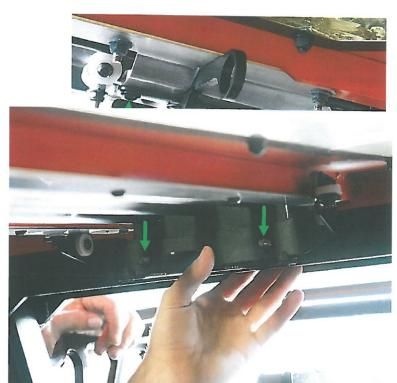
roller brackets onto the rails and onto the screws by overlapping the smaller bracket onto the larger. *They would have come pre-assembled that way.* Do not tighten the screws fully yet, leave them just a little snug. Test the rolling action and make sure the rails run evenly through the bearings. At this point you can release the spring-loaded bearings that you locked out earlier on the outer rollers.
