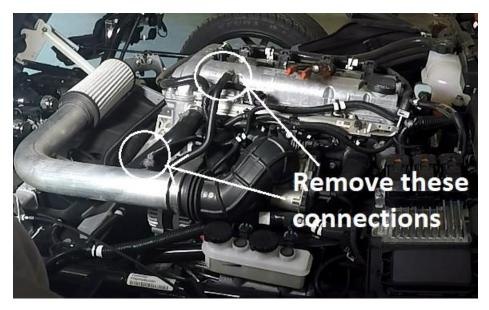
Step 2. Loosen Clamp screw collar mounting clamp at point over Intake manifold. Twist, rock and remove and let sit for now.
