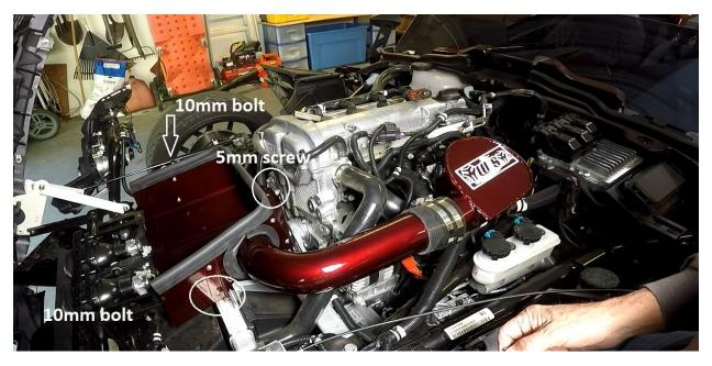
Step 9. Install Filter over the Inlet Pipe in Cage area. Slip Clamp over filer neck and slip filter over Pipe.
