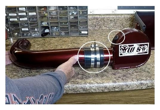
Clamps should be loosely installed over collar on Round Cage.
