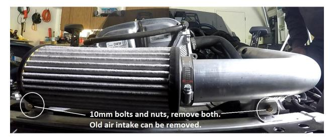
Step 4. All connections should be removed. Remove old Air Intake System as one unit.
