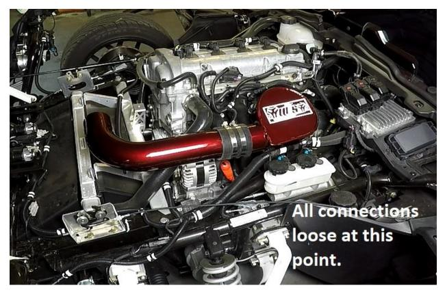
Step 8. Install Air Input Cowling. There are two 10mm bolts at the front and a 5mm allen screw at the back of Cowling. Front of Cowling must be inserted under the headlight supports and a certain amount of pulling and tugging will be required to get all bolts and screws to align for all connections. Tipping up from rear will aid in getting front 10mm bolts into position.
