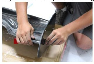
Step 2: With the (4) M8 1.25x30 Hex Bolts, secure elongated brackets and the arms through the roll bar. Insure the arms are fully secured to the roll hoops.
