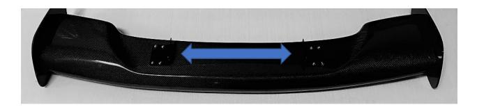
Step 4: Attach the wing to the bricks on the arms of the wing using (4) M8 – 1.25  $\times$  x16 Metric Hex Bolts and (4) M8 Flat Washers.
