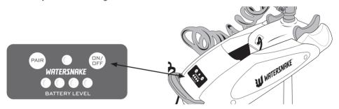
• The four lower LEDs indicate battery condition. They register as green or unlit, depending on charge remaining.
