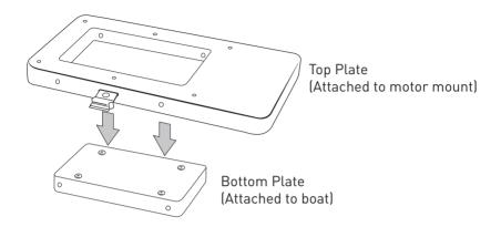
**4.** To lock both plates together, push the steel Locking Wire all the way into the holes shown here, so the Wire becomes secured by the metal clasp.
