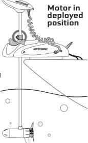
• Hold down the right-hand button (on/off) on the fascia panel on mount assembly until all the lights illuminate.
