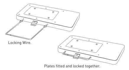
**NOTE:** A padlock can be used on the metal clasp of the quick release bracket to lock your motor to your boat.
